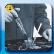
Measure electrolyte specific gravities and temperature!
