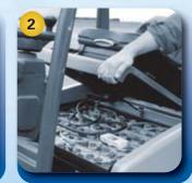
Remove battery cover! Leave vent plugs closed
