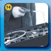
If insulation values are too high: Clean battery and extract liquid from inside the container!
