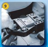
Visually inspect for damage Visually inspect all battery components for mechanical damage (particularly charging plug and cables).
