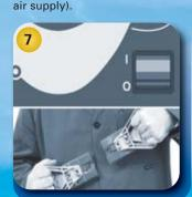
Switch off charger Switch off charger or check if charger has switched off. Disconnect clean battery if dirty! charger. Disconnect EC, if connected. Check final values if applicable
